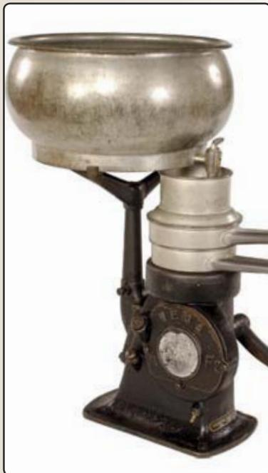
**Although most cream separators used in Canada were manufactured in North America, some were imported from Europe, like the Vega from Sweden (790394).**
